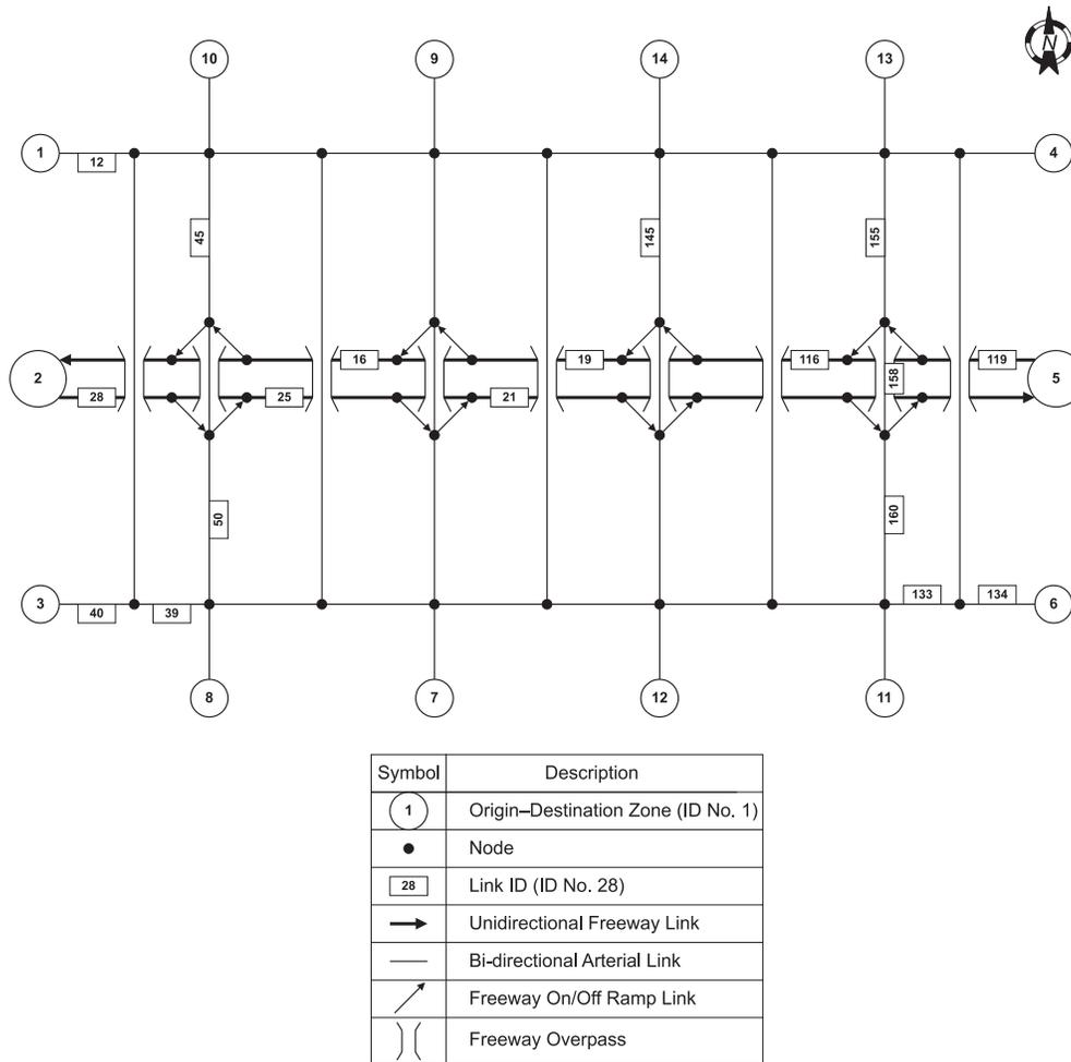
of a sample network used in the integration simulation model (M. Van Aerde 2000). The network represents a freeway-arterial system consisting of 56 nodes and 124 links. An east–west freeway is located in the middle of the network surrounded by arterial links with a total length of 6.4 km.
