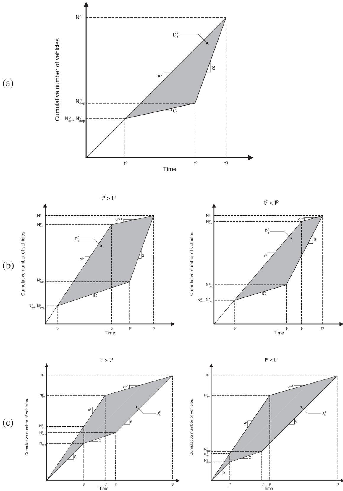
time period will occur after the incident queue clearance time. If the time required to clear the incident queue is long and (or) the accident occurrence time is close to the end of the period, the queue will extend to the next period. As a result, the uniform arrival assumed in case I is no longer valid and case II should be used.
